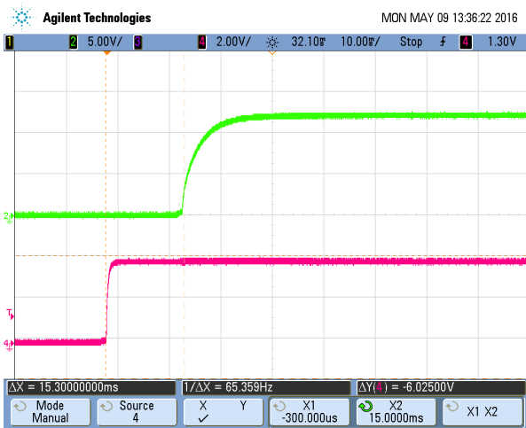
Turn-on transient at zero load current (10 mS/div, Top Trace: Vout, 5V/div; Bottom Trace: ON/OFF, 2V/div)
