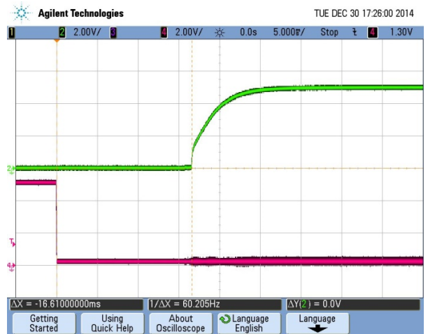
Turn-on transient at full load current (5 mS/div, Top Trace: Vout, 2V/div; Bottom Trace: ON/OFF, 2V/div)
