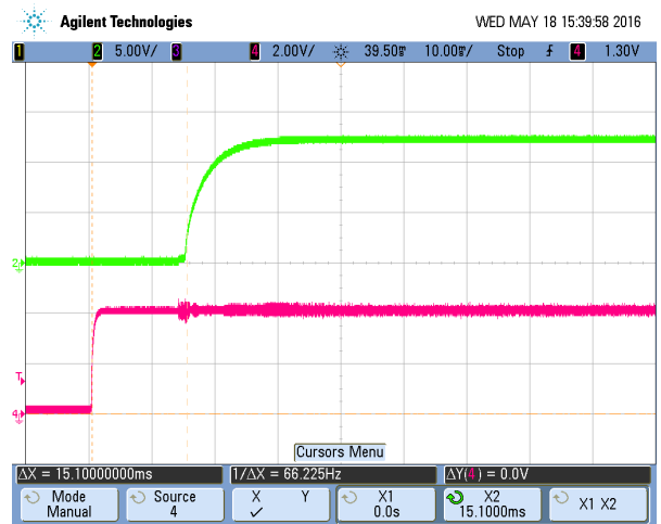
Turn-on transient at full load current (10 mS/div, Top Trace: Vout, 5V/div; Bottom Trace: ON/OFF, 2V/div)
