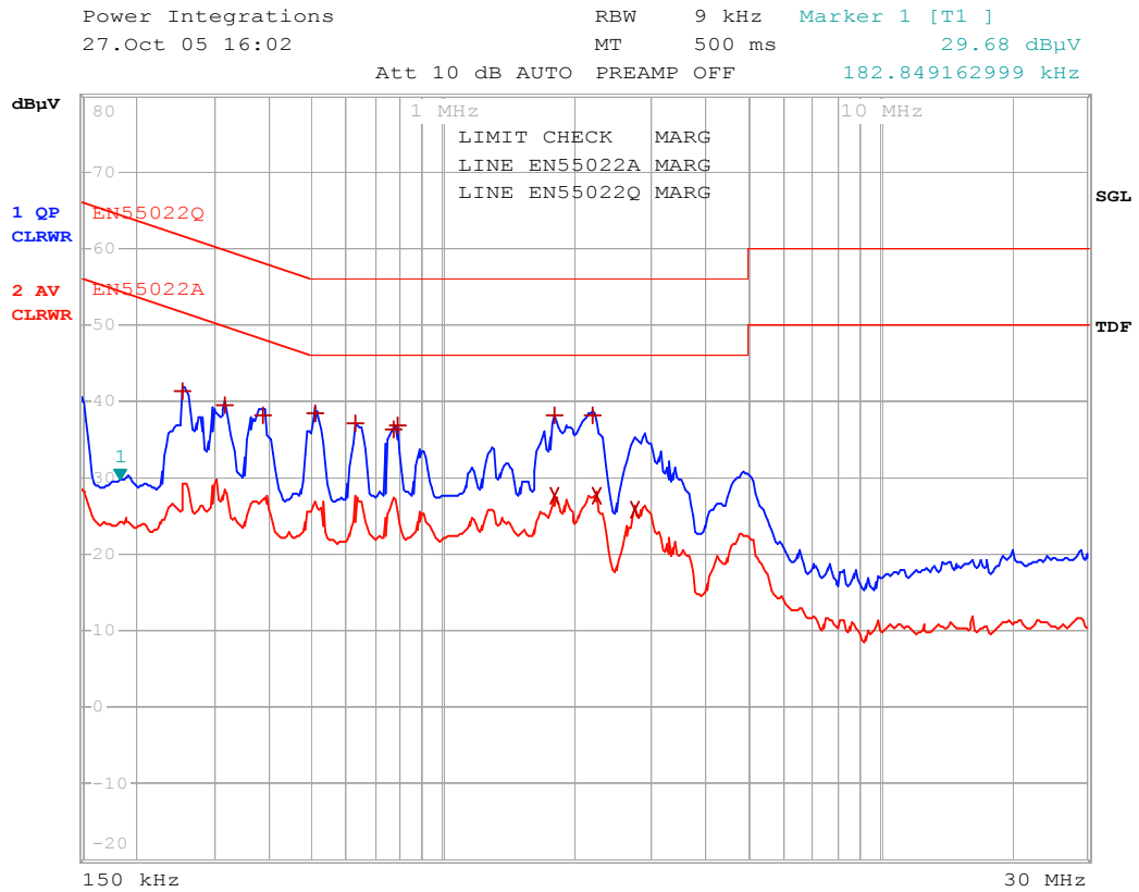
Figure 28 – Conducted EMI, Maximum Steady State Load, 230 VAC, 60 Hz, Artificial Hand and EN55022 B Limits.
