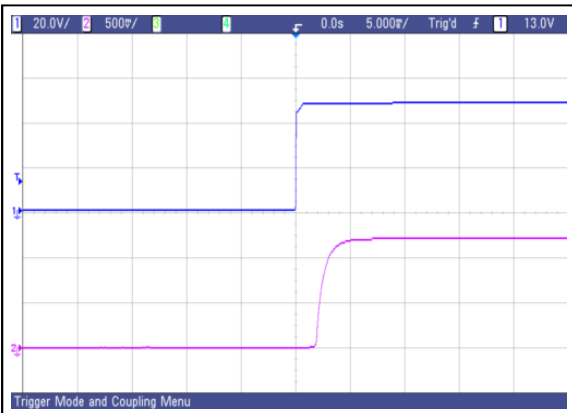
Figure 3: AVO50-48S1V2 typical start-up from power on
