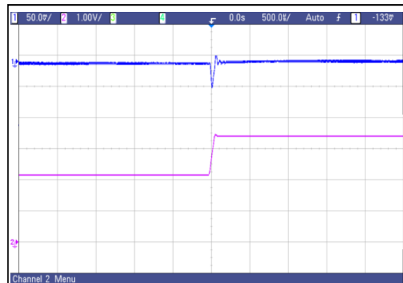
Figure 28: AVO50-48S1V8 Transient Response (500uS/div) 50%-75% load change, 0.1A/uS slew rate, Vin=48V
