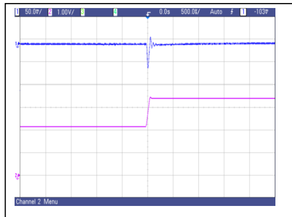
Figure 6: AVO50-48S1V2 Transient Response 50%~75% load change, 0.1A/uS slew rate, Vin=48V Ch 1: Vo Ch 2: Io
