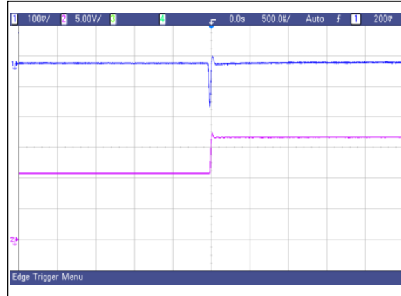
Figure 63: AVO50-48S05 Transient Response 50%-75% load change, 1A/uS slew rate, Vin=48V Ch 1: Vo Ch 2: Io
