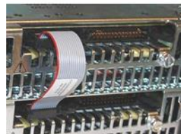
Shelf-to-shelf cable connection (part # CC848848952)
