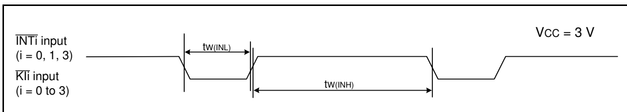
Figure 5.11 Input Timing for External Interrupt \overline{INTi} and Key Input Interrupt \overline{Kli} when V_{CC} = 3V
