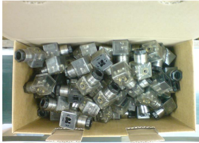
Figure 2 - Example of bulk pack mounted connectors
