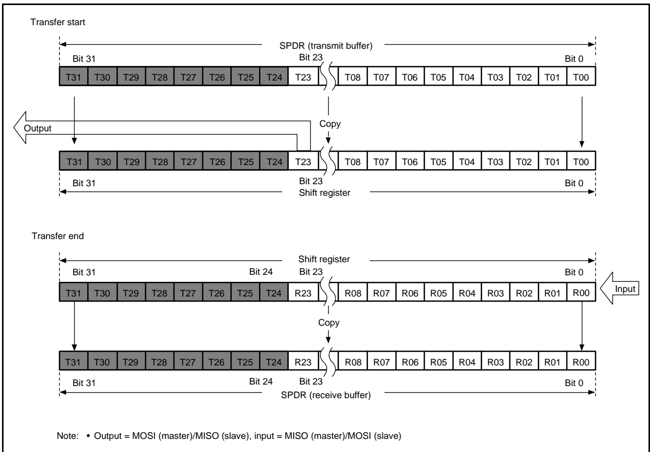
Figure 31.16 MSB-First Transfer (24-Bit Data, Parity Disabled)
